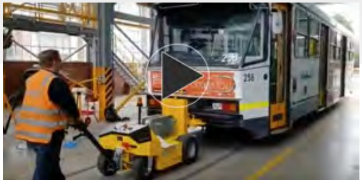
Movie shows pushing a 30 Tonne Tram with custom designed attachment
