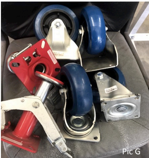
Non-marking elastic rubber tyres (RESILEX) provide quiet, smooth travel across a variety of surfaces.
